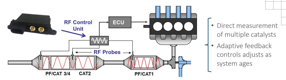
**CONCEPT:** Multi-function <u>*RF sensing platform*</u> to enable more robust and more efficient emission controls for gasoline, clean diesel and advanced low temperature combustion modes.
