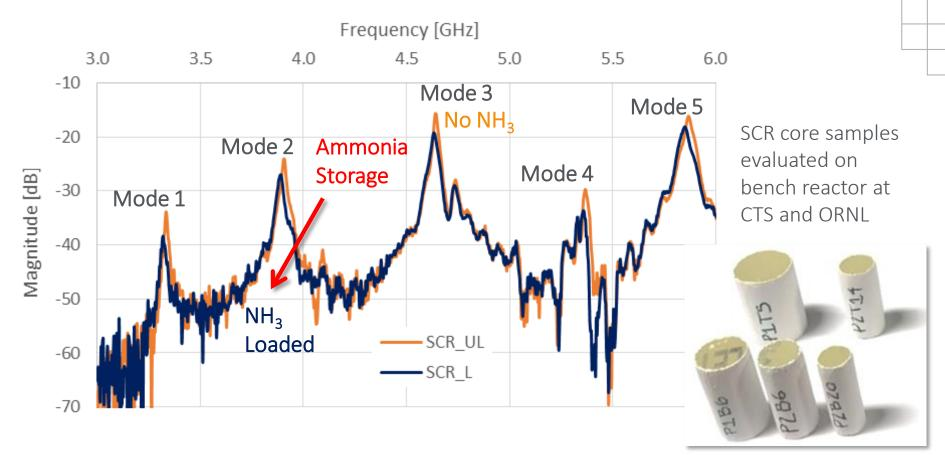
Catalyst Bench Reactor Testing Confirmed NH<sub>3</sub> Impact on RF Signal
