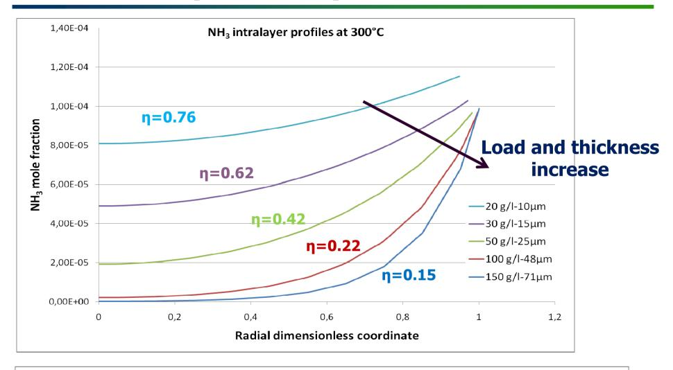
Internal diffusion control for higher washcoat loads/thickness
