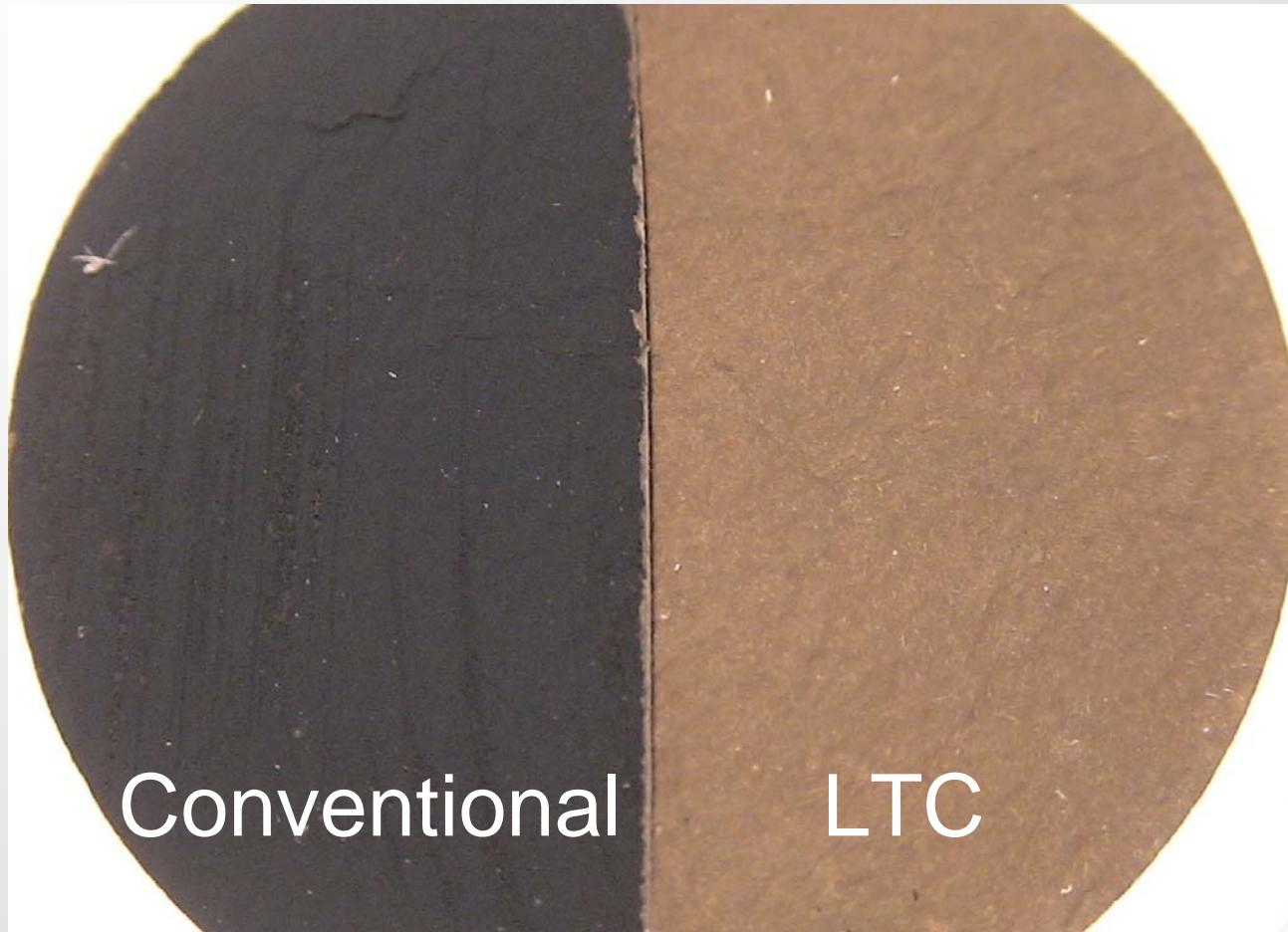
Color difference between PM from Conventional and LTC diesel combustion
