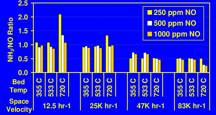
At 12.5K & 25K hr<sup>-1</sup>, optimum NH<sub>3</sub>/NO ratios for minimum NO<sub>x</sub>+NH<sub>3</sub> near 1.0 (or above), allowing high NO<sub>x</sub> conversions. At higher SV, optimum ratios << 1.0, limits conversions. > Kinetic limitations and the need to limit NH<sub>3</sub> slip
