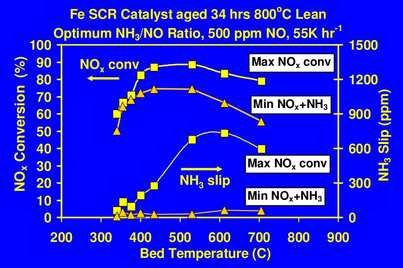
> At high space velocities, NH<sub>3</sub>/NO ratio producing maximum NO<sub>x</sub> conversion resulted in high levels of NH<sub>3</sub> slip
