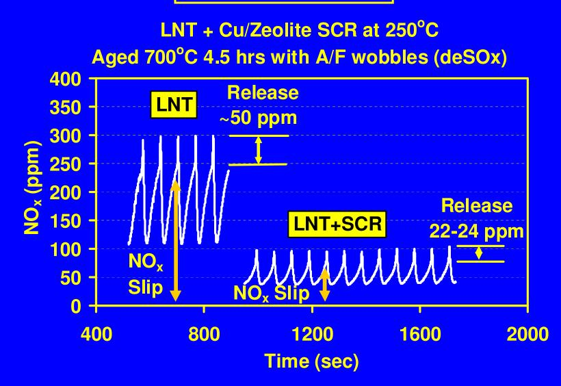
The  $NO_x$  release during purges and the  $NO_x$  slip during lean operation both decrease with SCR installed behind LNT.
