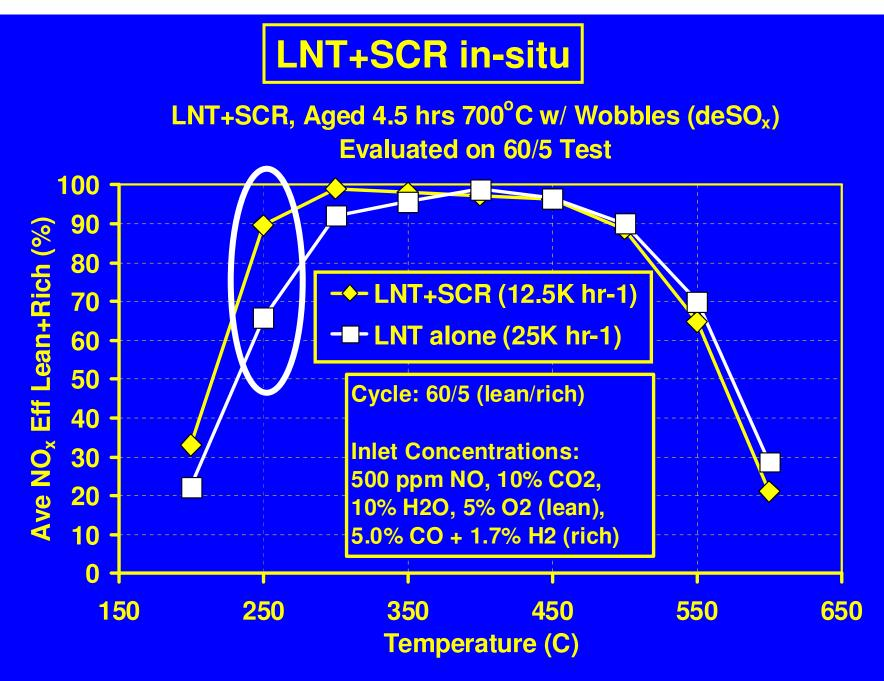
Cu SCR improves NO<sub>x</sub> conversion at 250-300°C.
