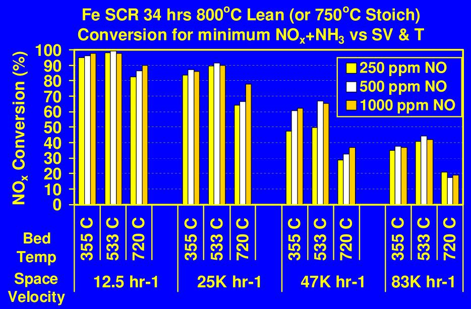
Largest SCR volume provided high NO<sub>x</sub> conversions and low NH<sub>3</sub> slip at all T and NO concentrations.
