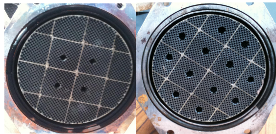
Drilled DPF to simulate different failure levels
