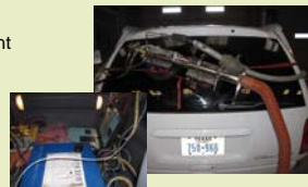
Two PEMS & other testing equipment including sample probes installed
