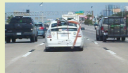
❖ In-use real-world testing with a GPS, a data logger and PEMS
