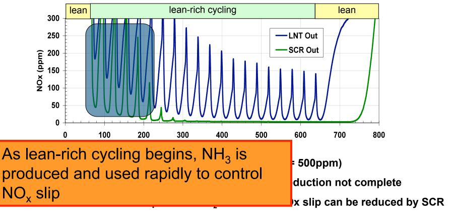
• Excess NH<sub>3</sub> stored by SCR enables more NO<sub>x</sub> reduction after cycling ends
