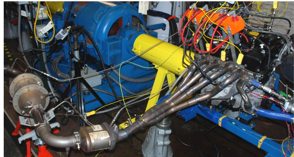
Final BMW 120i engine setup installed in ORNL engine dyno lab
